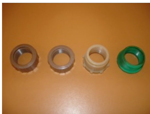
Photo 10 – Nuts made from PVC sleeves and reductions
