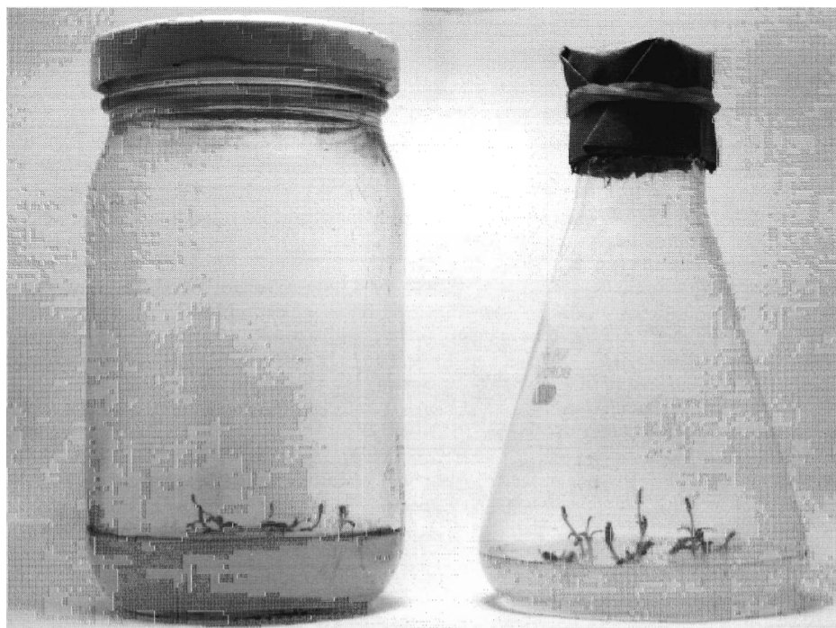
Figure 1: Sample 125 ml Erlenmeyer flasks topped with aluminum foil and paper sheets, and 200 ml food jars with metal twist-off closures from the in vitro germination experiments. Seedlings in the Erlenmeyer flask show advanced growth, possibly due to the greater light transmission allowed by the vessel and more efficient exchange of gases between the external and internal environments allowed by the type of closure.
